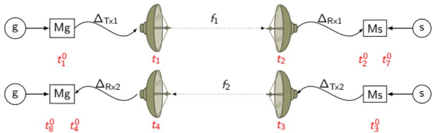
Two-way measurement setup ( $= 2 \times$  one-way)
