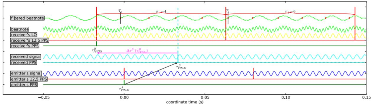
The system generates a beatnote between incoming signal and the local oscillator, then counts the number of zero-crossing for each sample.
