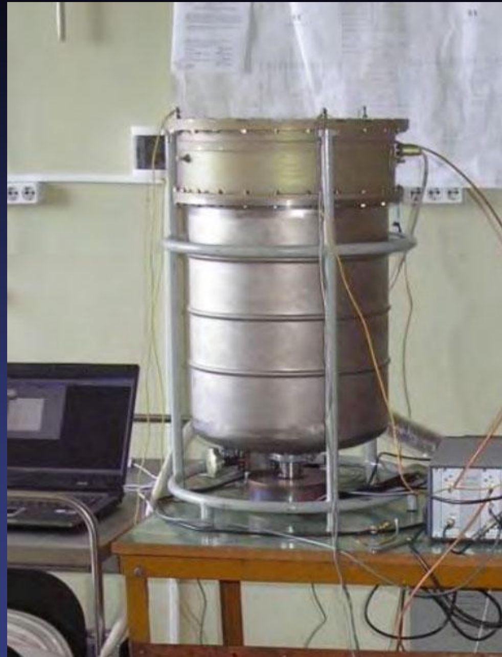
VCH-1010 Hydrogen maser frequency standard of the space radio telescope "RadioAstron"
