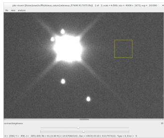
Homogeneous pixel-to-pixel noise of astronomical CCD
