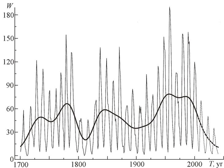
Fig. 2. (Solid curves) solar activity variations over the period from 1700 to 2006 (data from [1]) and (dashed curves) our predictions for the period from 2006 to 2040: (thin curve) 11-year variations, (thick curve) secular variations.
