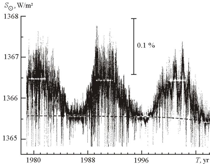
**Fig. 1.** Variations of the integral solar radiation flux over the period from 1978 to 2006 (the data were taken from [www.pmodwrc.ch/pmod.php?topic=tsi/composite/SolarConstant](http://www.pmodwrc.ch/pmod.php?topic=tsi/composite/SolarConstant)): (solid curve) 11-year variations, (dashed curve) secular variations. Individual upward and downward outliers are due to the passage of plagues or sunspots over the solar disk.
