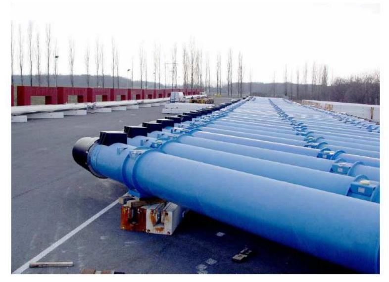
1232 superconducting magnets (before installation)
